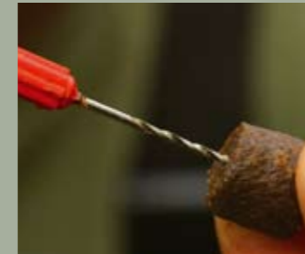
01 Use a fine, strong drill and make a hole through the centre of the pellet from end to end.
